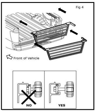
6) With tailgate down, slide mounting brackets into utilitrack. Be sure anchor plates are inserted into utilitrack and not outside of utili-track.
