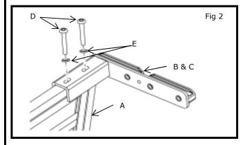
3) Loosely assemble mounting brackets (b or c)to divider (a) with bolts (d) and washers (e). Do not tighten.
